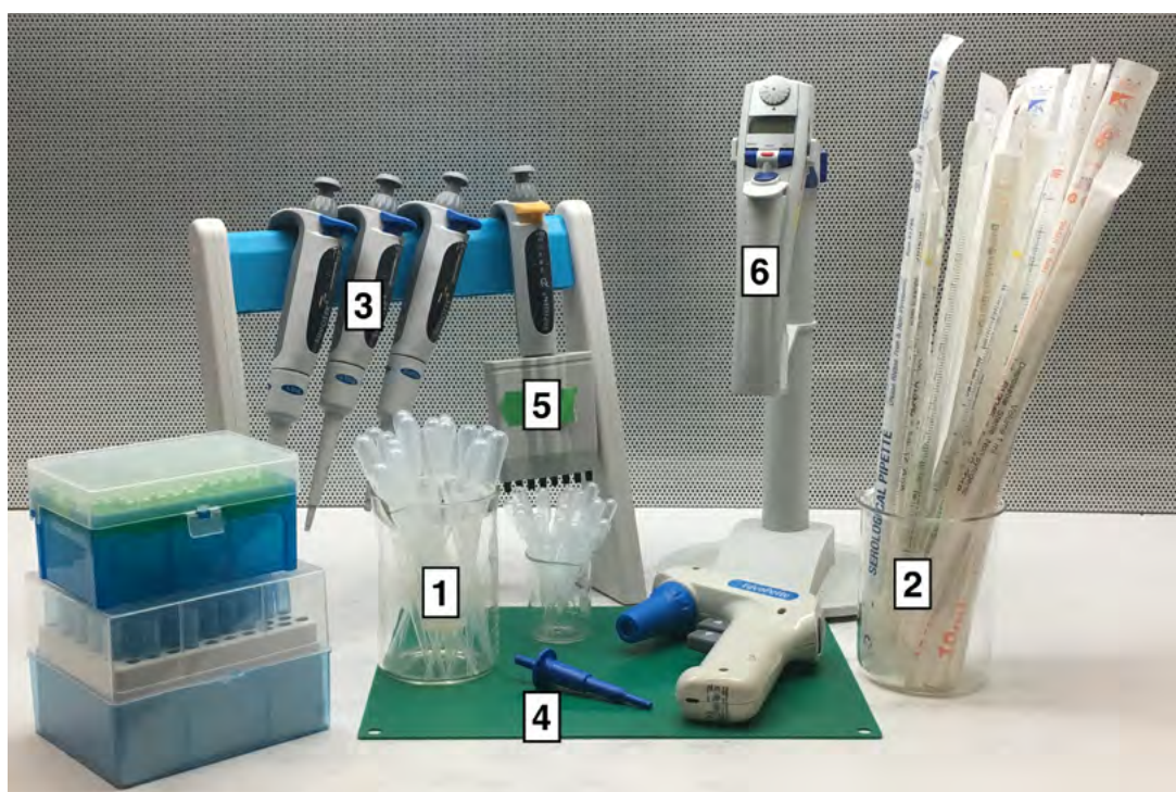
Figure 1: Common pipettes used in the lab. (1) Pasture pipettes, (2) Graduated pipettes, (3) Adjustable Micropipettes, (4) Fixed Micropipettes, (5) Multichannel Pipette, (6) Robotic Pipette.
