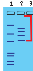
Figure 9: Measure distance migrated from the lower edge of the well to the lower edge of each band.
