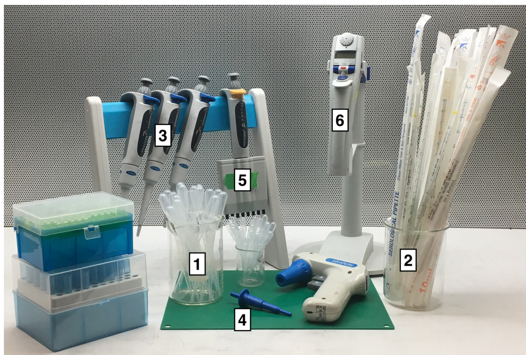
Figure 4: Common pipettes used in the lab. (1) Pasteur pipettes, (2) Graduated pipettes, (3) Adjustable Micropipettes, (4) Fixed Micropipettes, (5) Multichannel Pipette, (6) Robotic Pipette.
